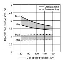
6-(2). Operate and release time (with diode) Tested sample: AGN2004H, 6 pcs.
