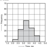
7-(1). Electrical life test (at rated load)
