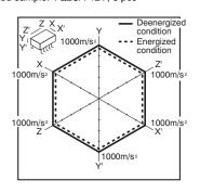
12.-(2) Malfunctional shock (latching) Tested sample: TQ2SA-L2-12V, 6 pcs.
