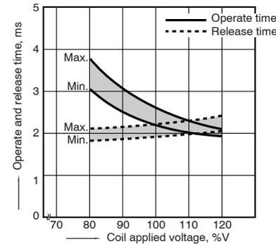
6-(2). Operate and release time (without diode)
