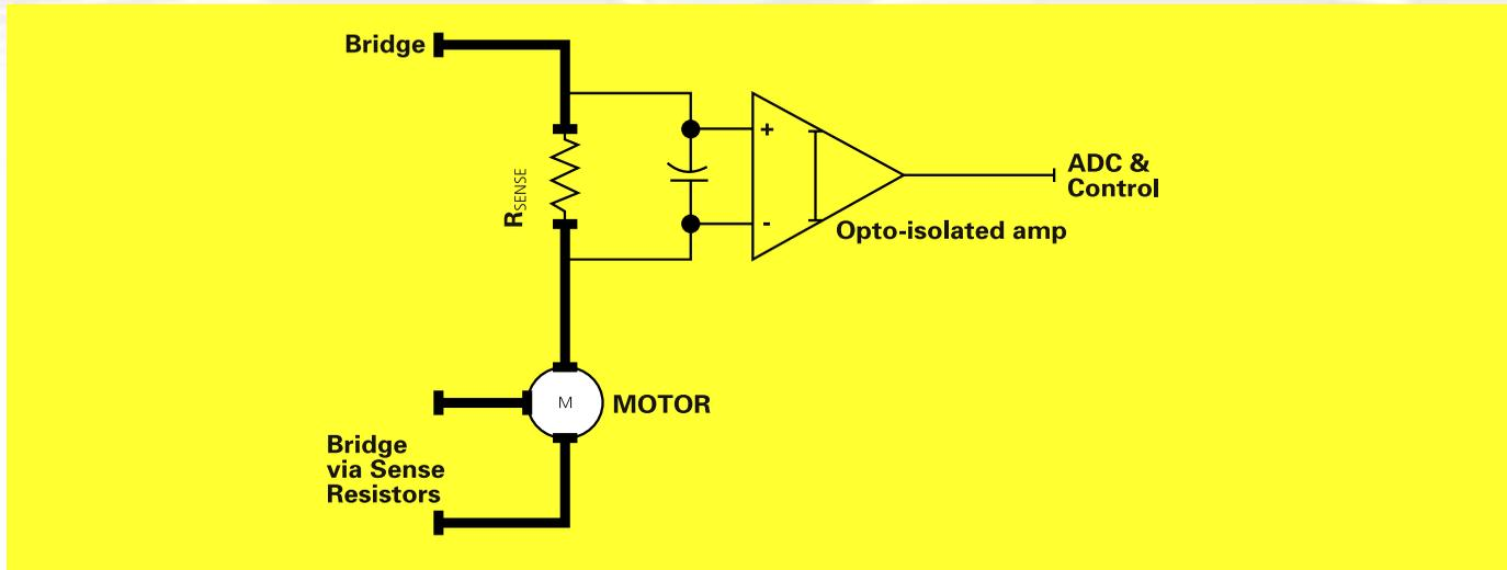
The important attributes in this case are the availability of values below  $10\text{m}\Omega$ , up to  $5\text{W}$  power rating with good surge withstand ability and low inductance. The ideal choice for RMS phase currents up to about  $20\text{A}$  is the OAR series, which is a pluggable, formed tape element resistor available in 1, 3 and  $5\text{W}$  ratings. The  $1\text{W}$  type is also available in surface mountable
