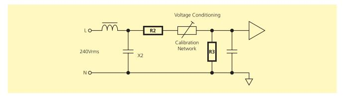
This is often achieved by means of a series chain of between four and eight MELF resistors, which provide the required stability and, in series combination, the required rating and pulse capacity. Depending on the cost of component placement and constraints on PCB footprint, a single element solution may be preferred. Data relating to both approaches is given below.
