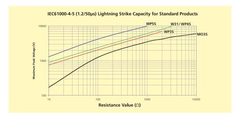
When calculating the peak voltage across the line input resistor it is necessary to subtract the clamping voltage of the MOV, typically 700 to 1000V, from the peak voltage applied to the circuit.
