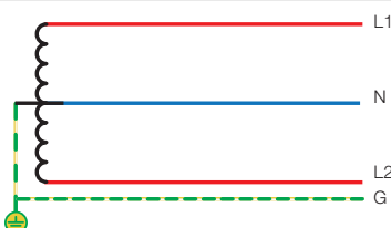
Grounded Wye 208 Y/120 V, 480 Y/277 V, 600 Y/347 V
