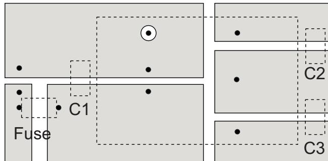
Input Fuse is recommended, but optional. Recommended fuse rating = double maximum input current, time delay type.
